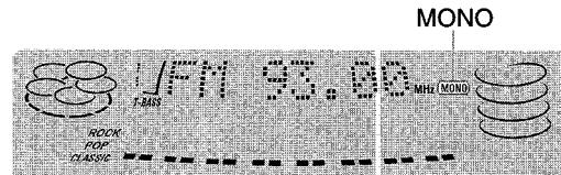
To restore stereo reception, press MONO TUNER on the remote control while pressing SHIFT so that "MONO" disappears.
